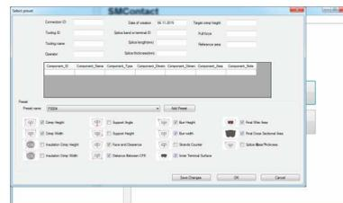
Viso 6.00 has 5 pre-stored sets of parameters (presets) which are to be examined during free measurement. They match the most common industry standards (VW
