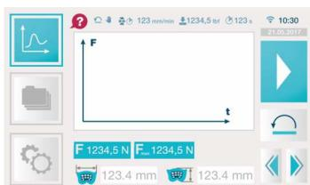
Measurement is done automatically in the selected mode. It is also possible to move the carriage manually if necessary. Results are visualized in real time on force-time diagram. Measurement modes: Break (destructive), Hold, Hold & Break (destructive).
