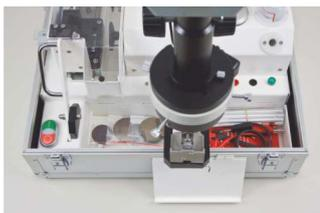
All necessary spare parts and consumables are included into supply kit: abrasive papers, cutting disks, etching pen inserts, electrolyte, crossline reticle, etc. They are also available
