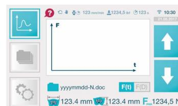
All connection parameters and measurement results are saved even if the test is aborted: selected mode, force-time curve graphics, crimp width and height, maximum force, and hold duration of maximum pull force (in Hold and Hold & Break modes).
