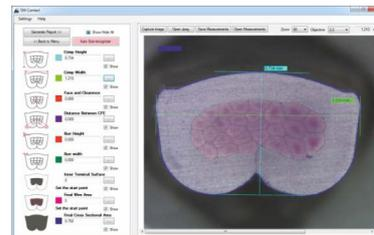
Captured image is measured with a help of special software – Viso 6.00. Operator chooses the parameters to measure, its reference values
