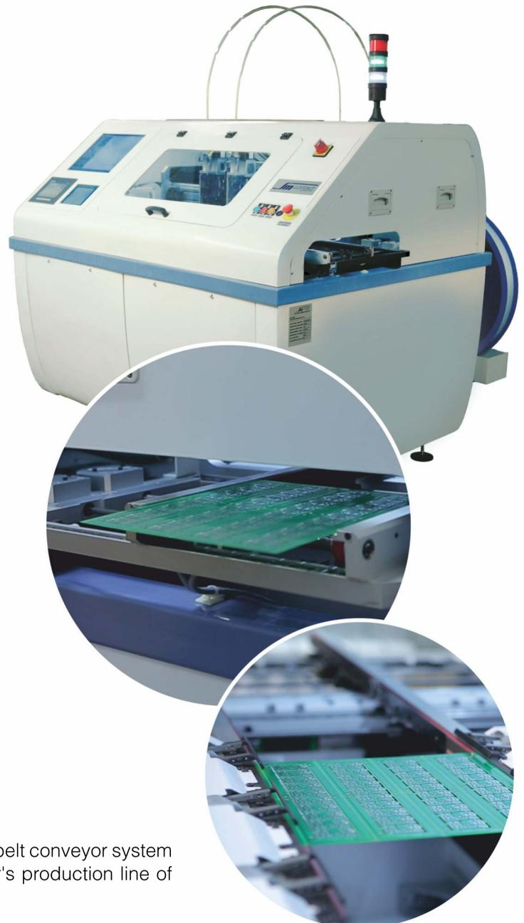
Pininsert 2200 CV is equipped with SMEMA compatible belt conveyor system to enable the integration of equipment to the Customer's production line of surface-mounted printed circuit boards.
